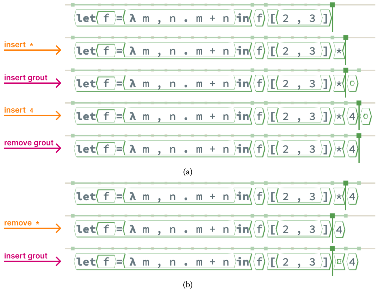
Figure 3.4: The grouter in action, invoked (in magenta) by ty1r after every user modification (in orange). We show the underlying tile structure rather than the default term structure for expositional clarity.
